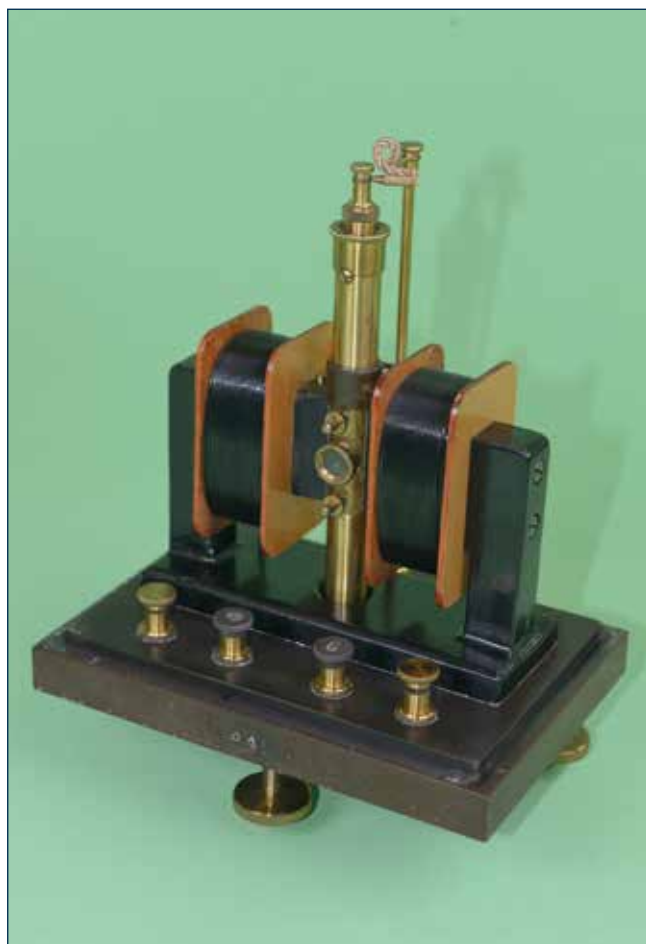
Fig. 1 Moll coil mirror galvanometer 1913 - V06652.
