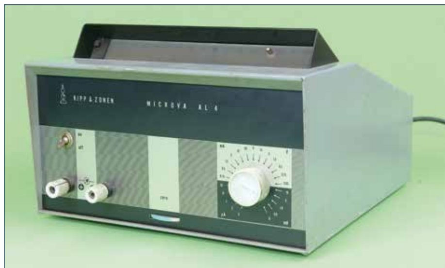
Fig. 3 Kipp Voltamp galvanometer, Microva AL4, 1959 onwards – V32155.
